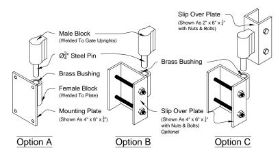
iDeal Barrel Hinge Custom To Fit Any Post Size Scale: NTS
